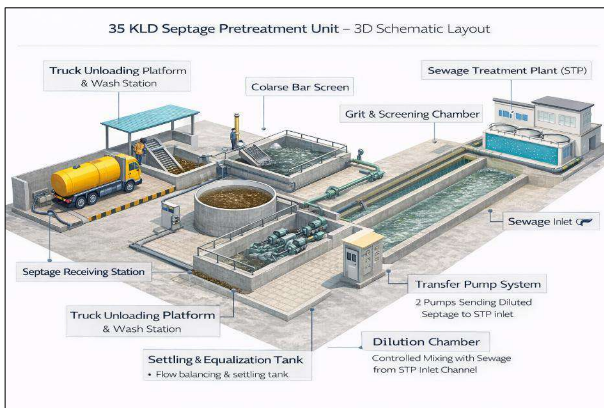
Figure 23 Schematic Layout of the Pre-Treatment Unit
