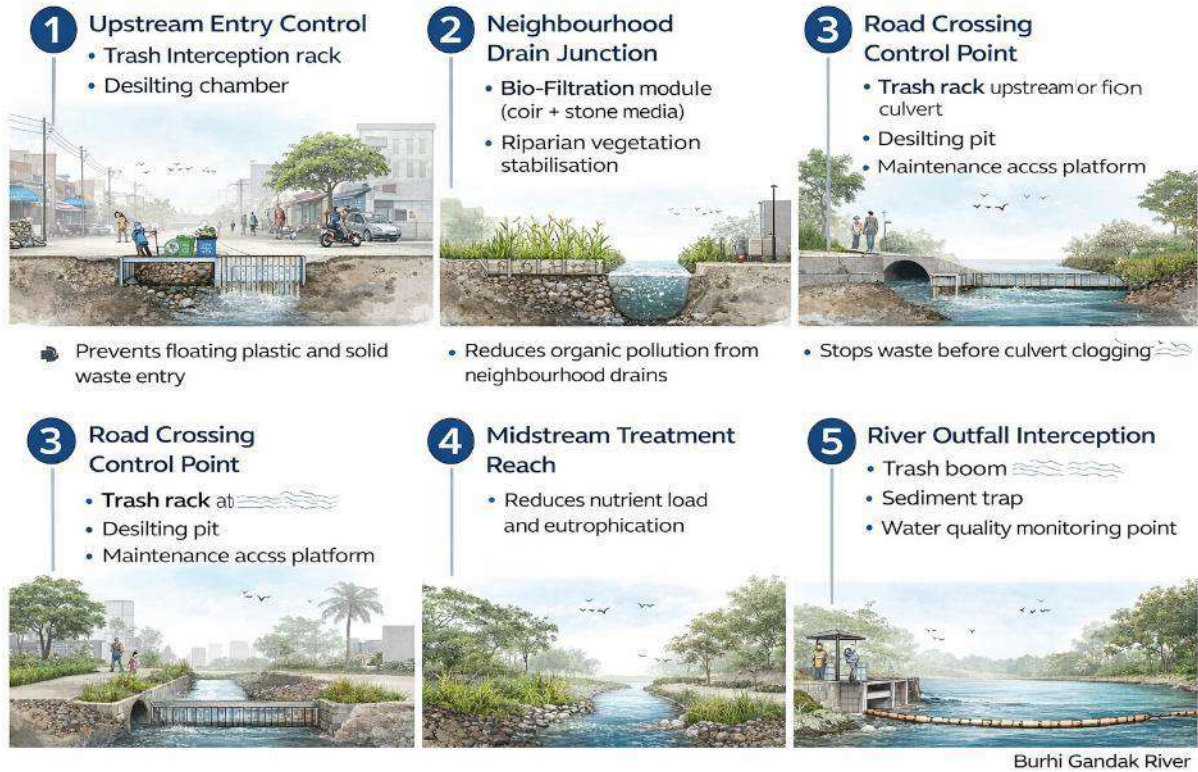
Figure 26 Sections for the 5 nodes of Chandwara Nallahs
